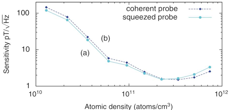
Figure 1: Sensitivity as a function of atomic vapor density in a single beam squeezed light enhanced magnetometer. Figure from Horrom *et al.* 2012 [5].
