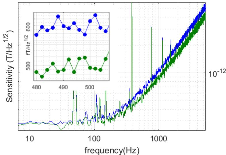
Figure 4: **Magnetic sensitivity spectra** for the Bell Bloom magnetometer probed with coherent (blue) and squeezed light (green). Taken from [38].
