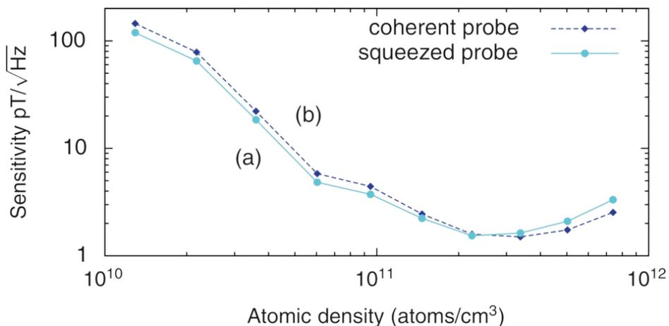
Figure 1: Sensitivity as a function of atomic vapor density in a single beam squeezed light enhanced magnetometer. Figure from Horrom *et al.* 2012 [5].
