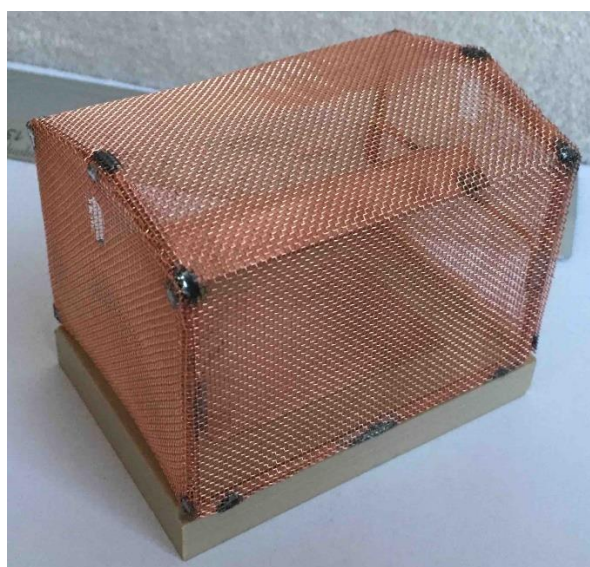
Figure 7: Detailed view at the electrode configuration for current detection. The configuration has been built in such a way that the detection of \text{NO}^+ ions is maximized whereas the photo effect is maximally suppressed.
